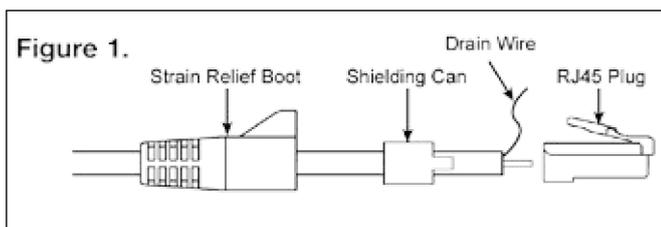
Prepare cable as you would for UTP assemblies. Place the boot onto the cable, followed by the metal can, as shown above.
