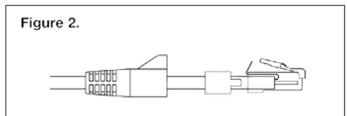
Terminate the RJ45 plug prior to fitting the shielding can. Bend the drain wire across the top of the RJ45 body as shown, trim if necessary.
